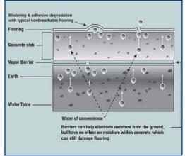
The first step is to conduct moisture testing. Substrate surfaces must be tested for moisture emission prior to starting the installation. Most manufacturers and flooring installation contractors recommend Relative Humidity probe moisture testing, as the results of this type of test are typically more accurate, reliable and consistent than other testing methods.
